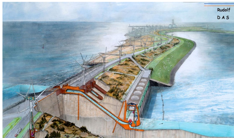
Figure 6. Cross section of Energy Island PSH.
